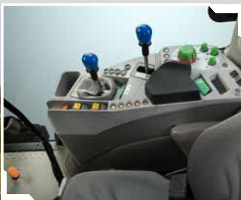
Mechanical cross lever to activate 4 hydraulic ways with the same control.
