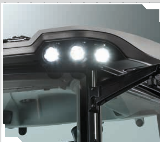
New roof design with up to 12 LED working lights.
