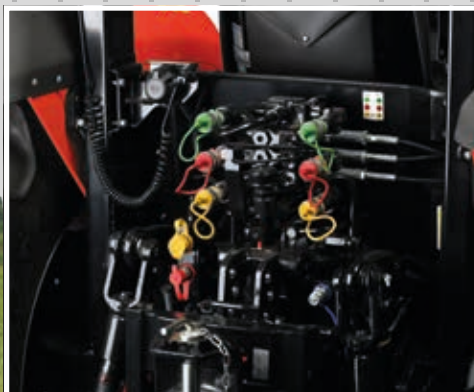
Up to 3 spool valves with flow regulator.
