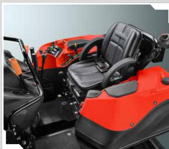
Comfortable driving station mounted on Silent-Blocks.
