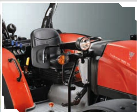
Rear mirrors installed in the front of the platform available as option.
