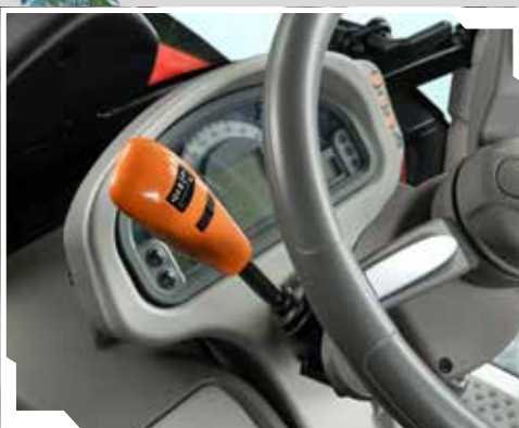
PowerShuttle with SenseClutch, Stop&Go and ComfortClutch available.
