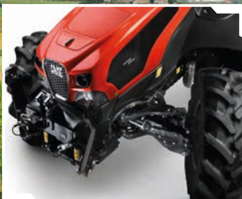
ActiveDrive independent front suspension.
