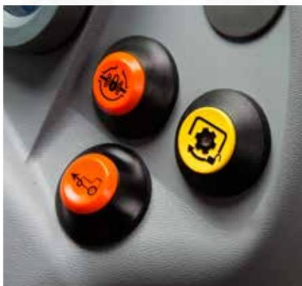
Explorer<sup>3</sup> TB tractors feature electro-hydraulically selected differential locks and 4WD as standard.
