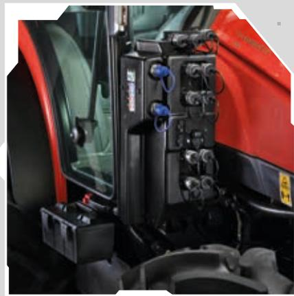
Up to 5 high-flow rear spool valves and 1 free return. Power. Beyond and hydraulic trailer brakes as option.
