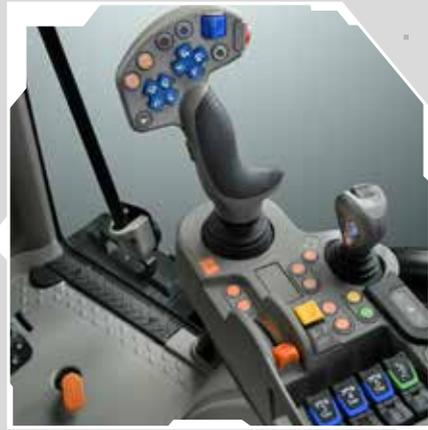
Easy to operate rear and mid-mounted spool valves thanks to proportional controls. The controls can be freely assigned through InfoCentre<sup>Pro</sup> settings.
