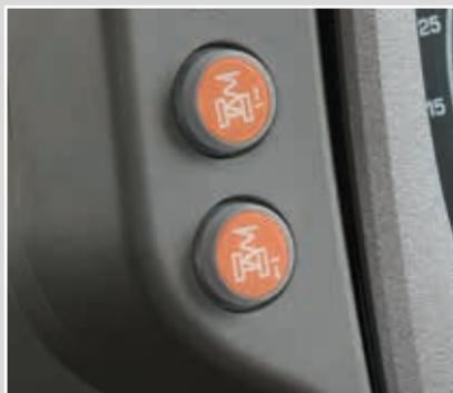
New: two dedicated buttons to manually adjust the position of the front suspension to facilitate maintenance operations and to ensure easy coupling maneuvers of the front equipment.
