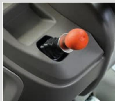
All SAME Frutteto CVT tractors are equipped with all-wheel braking and a Hydraulic Parking Brake (HPB).
