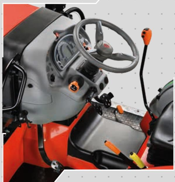
In order to cater the needs of all orchard growers, the tractors of the new Frutteto family are offered with two different platform height variants. The higher platform is able to accommodate big rear tyres, up to 28", while the lower one has been designed keeping in mind the need of the orchard growers which needs a tractor as low as possible.
