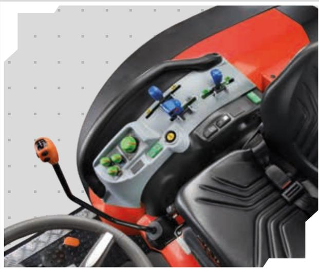
The hydraulic system is designed to provide maximum efficiency and reliability. It features a dedicated distributor for the front lift, ensuring precise control and modulation of movements. The system is integrated into the front of the tractor, minimizing the overall footprint.
