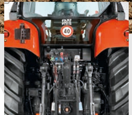
Equipped with a dedicated 120 l/min Load Sensing.
