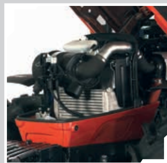
The monolithic bonnet in sheet metal makes the access to the engine always easy.
