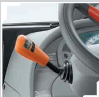
Hydraulic modulation for PowerShuttle sensitivity.
