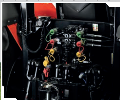
Up to 3 spool valves with flow regulator.
