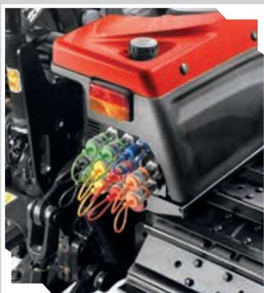
Up to 10-way rear hydraulic distributors.
