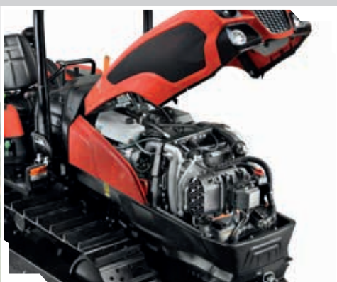
3 cylinder FARMotion engine.
