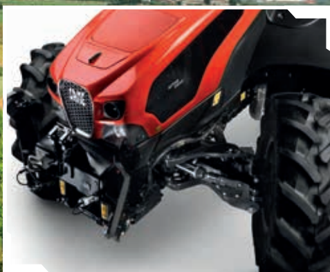
ActiveDrive independent front suspension.
