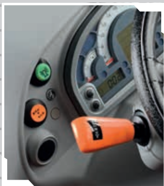
Hydraulic PowerShuttle with Stop&Go.
