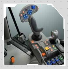
Easy to operate rear and mid-mounted spool valves thanks to proportional controls. The controls can be freely assigned trough InfoCentre<sup>tro</sup> settings.
