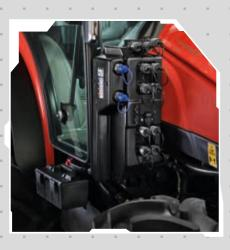
Up to 4 high-flow mid-mounted spool valves and up to 3 hydraulic ways duplicated from rear and 2 free returns.
