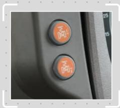
New: two dedicated buttons to manually adjust the position of the front "suspension to" facilitate maintenanace operations and to ensure easy coupling maneuvers of the front equipment.
