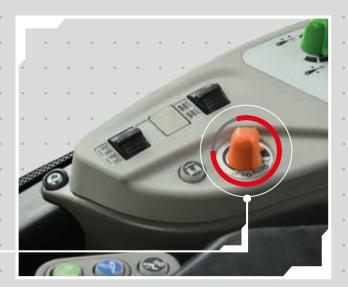
A specific dial lets the operator select within a range from "ECO" engine management mode, for minimised fuel consumption, to "Power", for maximum power.
