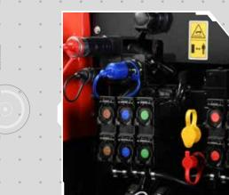
Up to 5 high-flow rear spool valves and I free return. Power Beyond and hydraulic trailer brakes as option.
