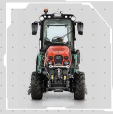
The high number of hydraulic connections (up to 21) allows the installation of combination of implements (front, mid and rear mounted). Frutteto CVT S can be equipped with a shaped fuel fank allowing the installation of mid-mounted implements while keeping the overall width of the tractor less than 13m.
