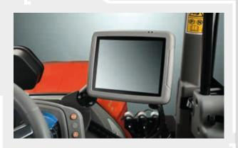
The Frutteto CVT, Frutteto CVT S and Frutteto CVT V can also be equipped with the 8" iMonitor, installed on the right hand corner of the dashboard with an adjustable mount.
