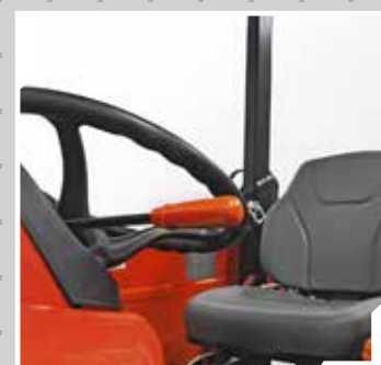
Shuttle lever conveniently located under steering wheel.
