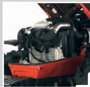
The monolithic bonnet in sheet metal makes the access to the engine always easy.
