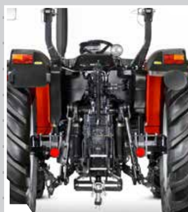
Rear lift capacity up to 4200 kg.
