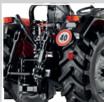
Mechanically controlled rear lift available in two versions.
