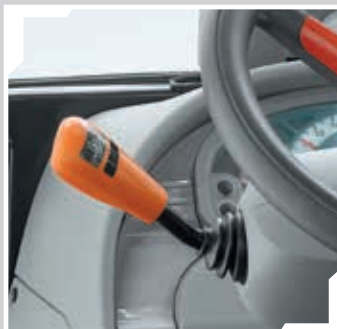
Hydraulic modulation for PowerShuttle sensitivity.
