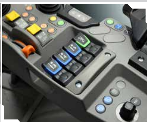
Electronically controlled hydraulic distributors.
