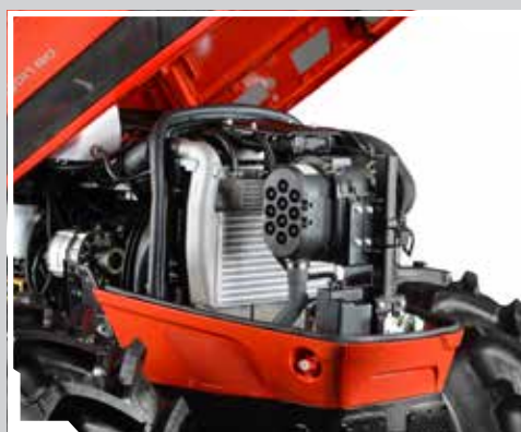
FARMotion Stage III B 3-cylinder engines:
