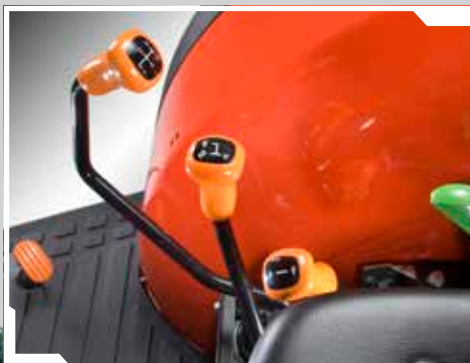
Transmission controls with side handles.
