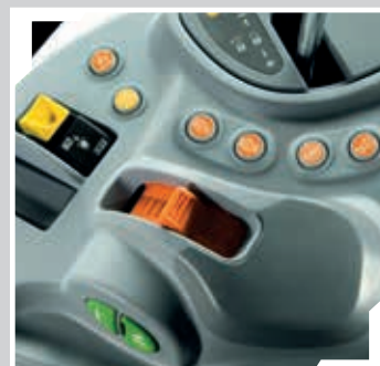
Electro-hydraulic controls for the main functions.
