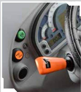
Hydraulic reverse shuttle with Stop&Go.
